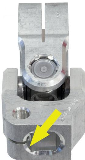
*Old joint (steering spindle) without recess*
