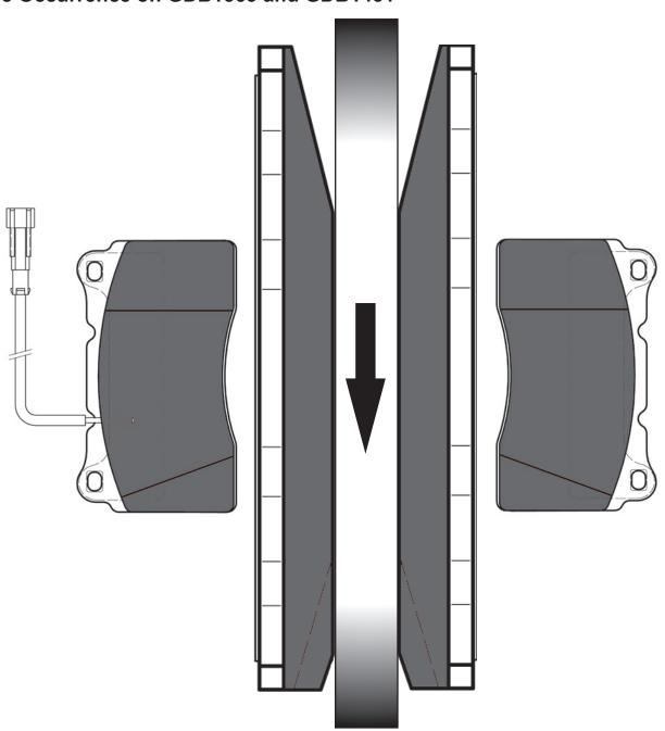
GDB1363 and GDB 1431 are chamfered on one side. The reason for this is to minimise noise. The arrow indicates the disc forward rotation. If the Brake Pads are not fitted as shown above, noise will occur. To ensure the correct fitment in future TRW will print indicator arrows on the back plate.
