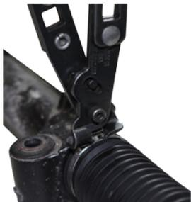
Depending on the type of clamp enclosed, make sure to use the respective appropriate special pliers!
