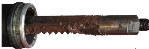
For bellows, do not use standard hose clamps or cable ties. Thereby, the bellows can cast pleats. Water and contamination can ingress through these.
