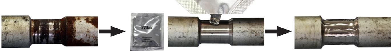
Before the bellows are installed, the sealing surfaces must be cleaned and free of corrosion. To optimize the sealing, apply enclosed silicone grease to the sealing surfaces of the tie rods. Always use the new accessories supplied.
