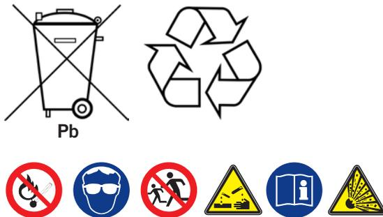
Labelling might vary due to application and dimension of the Battery. The manufacturer, respectively the importer of the batteries shall be responsible for placing the symbols (a minimum size is specified). In addition, consumer/user information on the significance of the symbols may be attached.
