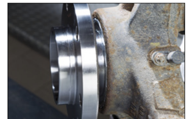
Image 3: The locking ring must lie flush with the steering swivel
