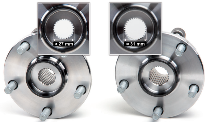
Figure 2: The diameter of the CV Joint spline is different
