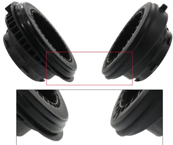
Fig. 1: Strut support with splash guard (left) and without (right)
