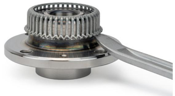
Image 2: The sensor ring must be removed if the wheel bearing is installed in vehicles without ABS. This can be done using a tyre lever, for example.
