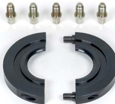
The clamps ensure firstly that the snap ring is held in position during installation. They secondly guarantee that the forces are routed via the outer ring during the pressing-in process
