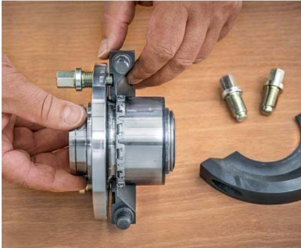
Wheel bearings are safety-relevant vehicle components, which are manufactured to very tight tolerances using high-precision machinery. That makes it all the more important to remember this during repairs and to work carefully.
