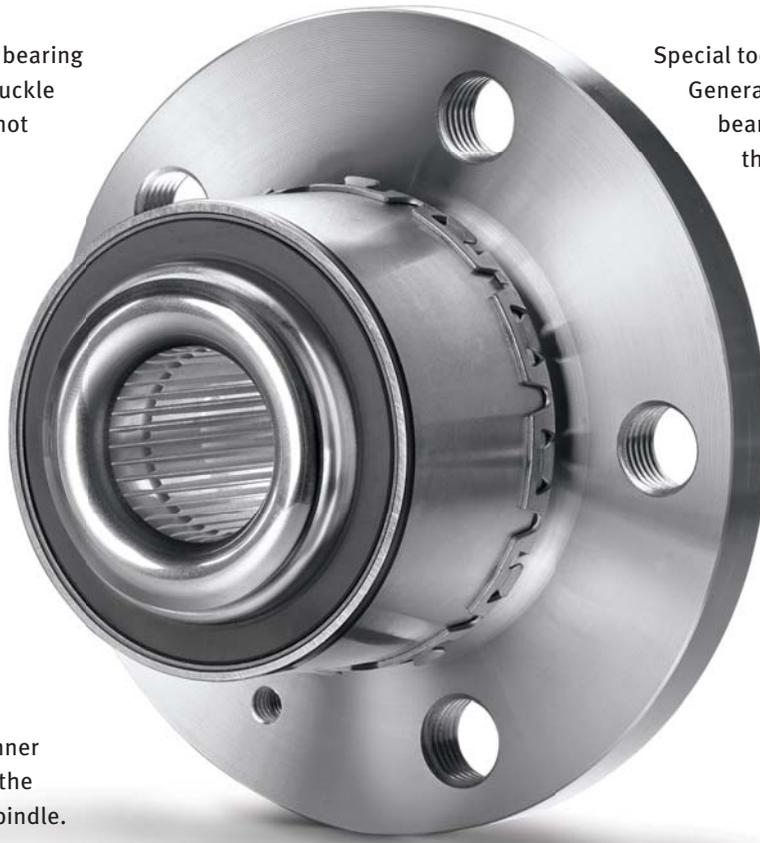
Special tools are vital for Generation 2.1 wheel bearings. There are two things to remember during this process; firstly the pressing force must be applied via the outer ring, and secondly the snap ring must be held in position so that it ultimately engages into designated groove in the steering knuckle.
