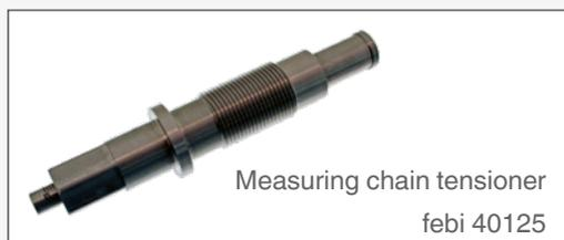
The measuring chain tensioner has a graduated scale from 55 to 85. If all chain drive components, e.g. chain tensioner, chain, guide rails and sprockets, are in perfect condition, the measuring chain tensioner should indicate a value of approximately 62.5.
