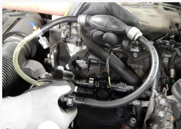
Figure 2 Fuel system bleed tool installed and ready to use
