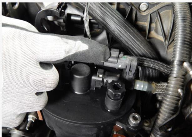
Figure 1 Fuel temperature sensor connector
