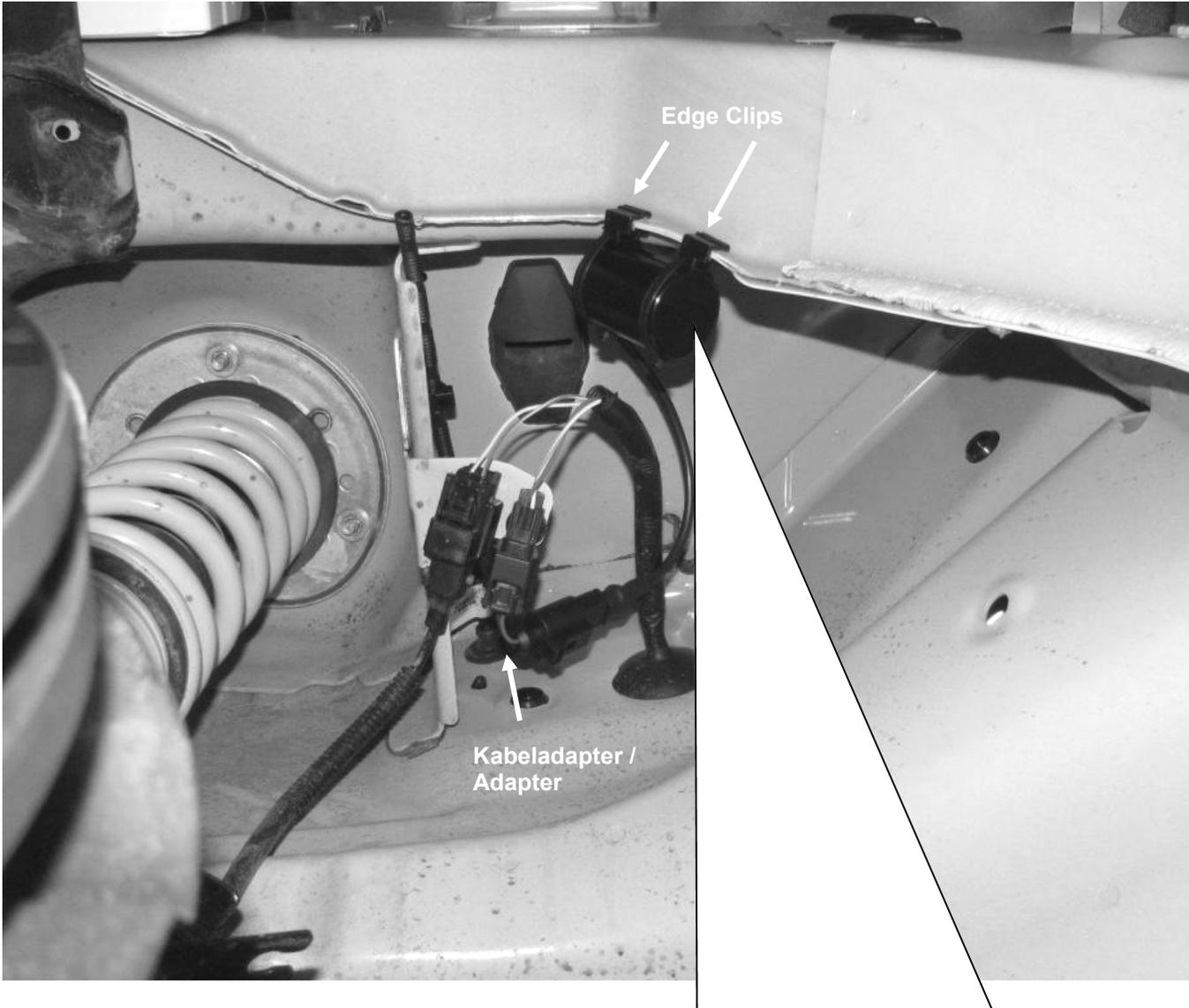
Montageort VA Elektronik Satz / Assembly site front axle electronic kit
