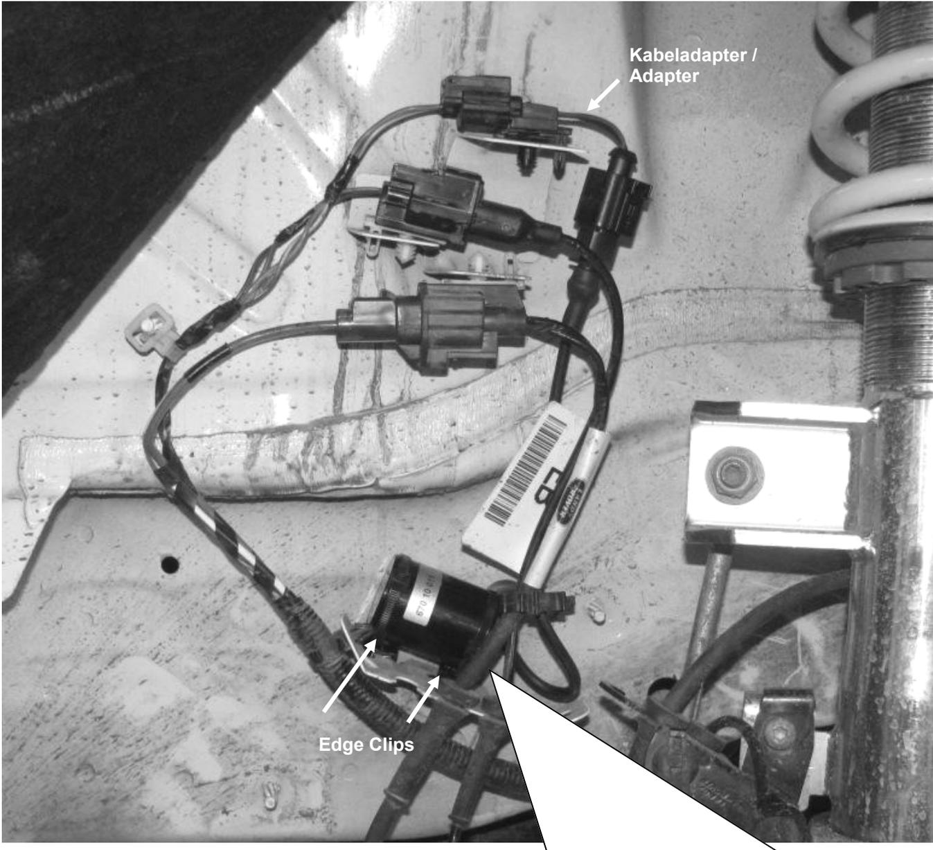
Montageort VA Elektronik Satz / Assembly site front axle electronic kit
