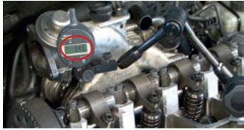
> Turn the lobe axis until the injector lobe reaches its maximum height, then the injector will be powered.
