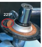
➤ Loosen screw 225° using a goniometer.
