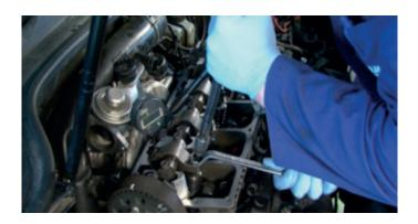
> When this point is reached, loosen the nut and tighten the screw in the rocker and a resistence is visible.
