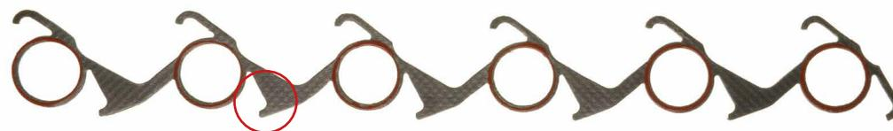
In case of cutting out the intake manifold gasket, it must be done following the shape of the gasket bores, as shown in the following image:
