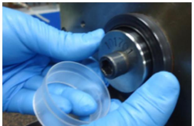
Assembly of the PTFE seal in its housing
