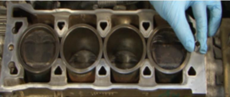
*Do not turn the crankshaft once you remove the tools to pin up liners.*
