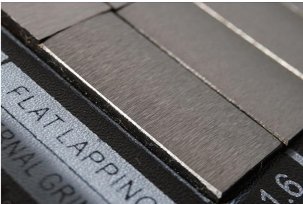
The **maximum roughness** ( $R_z$ ) is defined as the arithmetic mean of the height between the lowest highest points of the surface. It is measured in **micrometers** ( $\mu\text{m}$ ) and is used to indicate the depth of the deepest grooves in the surface.
