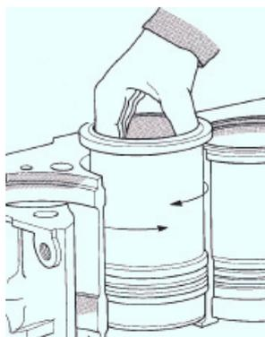
3. Using a dial gauge, **measure the height** between the cylinder liner projection and the block at the 2 points indicated. Always on the camshaft side.
