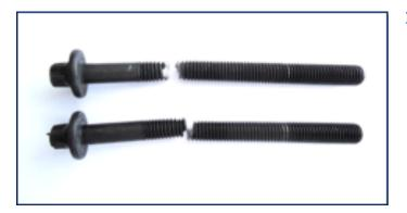
An over-tighten or reusing the bolts, may lead to an incorrect sealing of the cylinder head gasket or even the bolt breakage in the area where tensions are critical.
