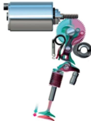
*All **intake valves** are linked to an axis actuated by an electric engine electronically controlled, which changes position depending on the engine requirements. Depending on the axis position, **the actuating lever will rest in different positions** on the valve rockers, which will open when the lever receives the camshaft movement at a certain height to allow the mixture.*
