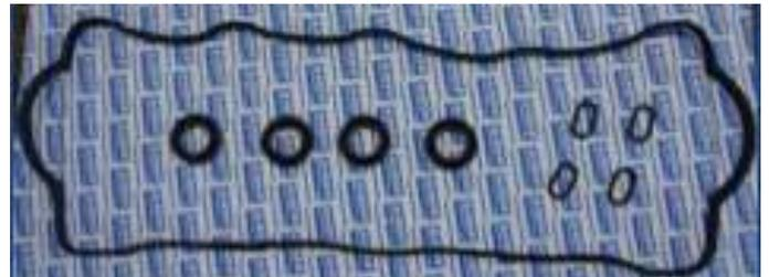
2 For the installation of the new injector oil seals will **use the special tool that allows us to put them level and positioned correctly**. Then place the gasket in housing without applying any sealant in this section.
