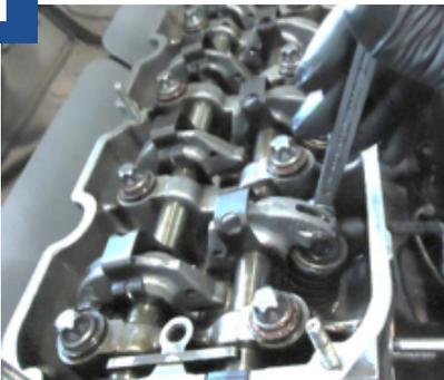
*Loosen the fixing nut of the eccentric washer of the rocker to be adjusted.*
