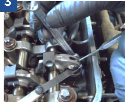
*Tighten the nut for fixing the eccentric washer in the correct position while the gauge is introduced between the rocker and the valve head.*
