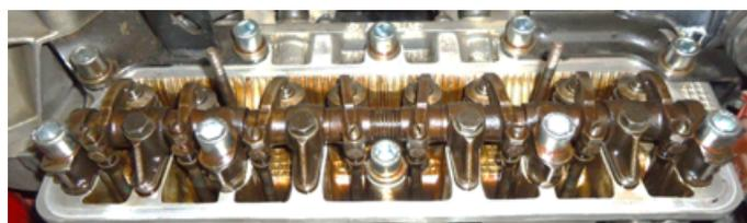
**2.** Loosen the lock nut to release the rocker arm adjusting bolt and act on it until we get a considerable gap between the rocker and the valve.
