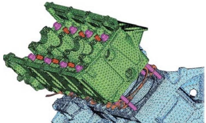
Nowadays, the use of angular tightening bolts is widespread because they adapt to the specifications of the manufacturers of modern mechanics. This kind of bolts must be replaced always when repairing the engine.
