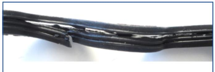
It should be considered that the tightness of these type of gasket usually is between 8-12Nm, and if the screws are tightened without using a dynamometer, it's probable that its reaching the 25Nm easily without realizing it.
