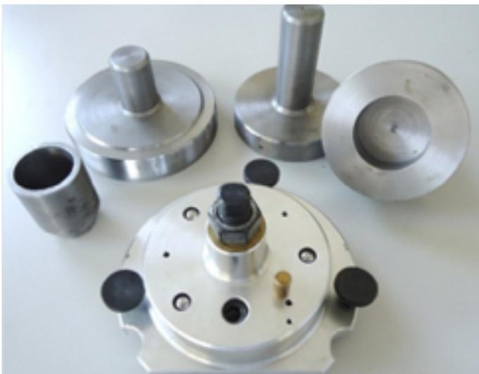
The assembling it must be done **by an adequate tool** that allows the oil seal to be inserted into its housing at the same time throughout its diameter, in this way, we can ensure that the oil seal is perfectly perpendicular to the axis where it is mounted, making sure that the internal lip acts in the same way on the entire surface of contact with the shaft.
