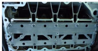
The reason that Land Rover recommends replacing the oil duct when ordering the cylinder head gasket, it's not specific.
