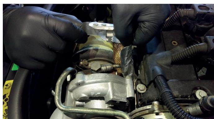
**3** Unscrew the **3 nuts** which connect the turbocharger to the catalytic converter and remove the bracket of the catalyst to the exhaust line.
