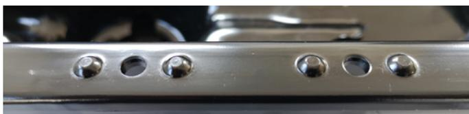
Detail of the **stamping protrusions** of a new oil pan
