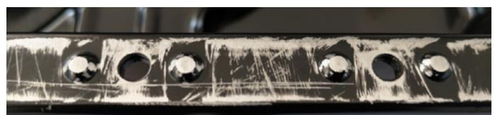
Detail of the **stamping protrusions** of an old and used oil pan
