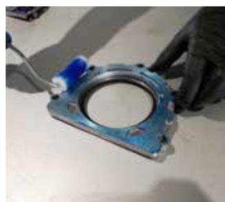
**4.** Join the components to be sealed **before 15-25 minutes** after the sealing application.
