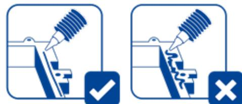
It must be applied sealant **bordering** all the holes and the entire perimeter, as indicated in the following pictures:
