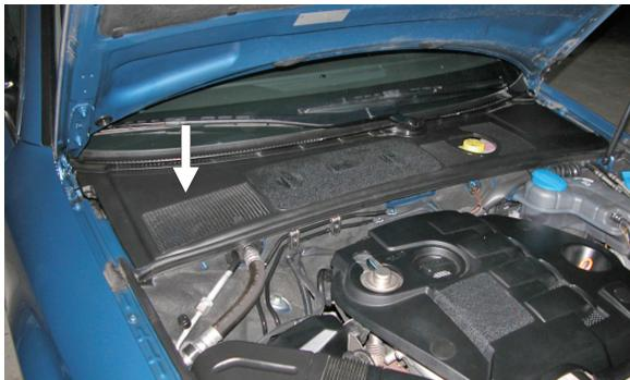
**EN** Pollen filter is located behind the engine chamber. Remove the screen under the windshield
