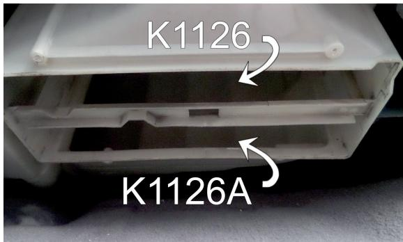
**(EN)** There are two separate filter assembly chambers
