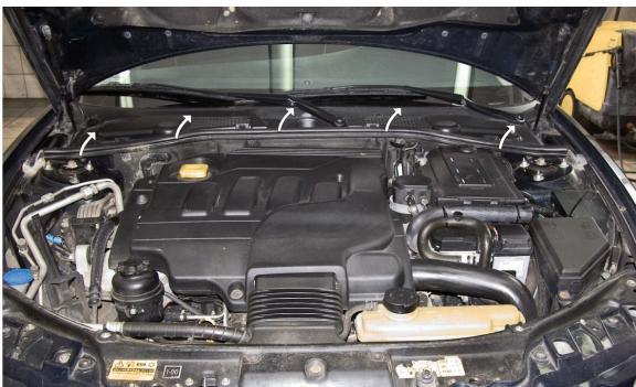
**(EN)** Remove the rubber seal
