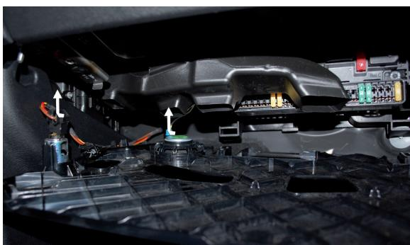
(EN) Disconnect the electric circuit
