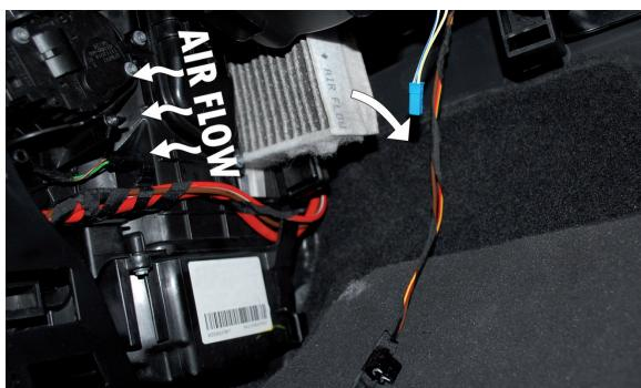
**(EN)** Carefully remove the first filter
