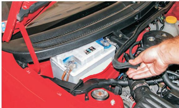
(EN) Remove the rubber seal
