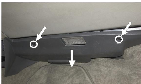
(EN) Loosen the screws and remove the upper wall of the locker. Remove the upholstery panel
