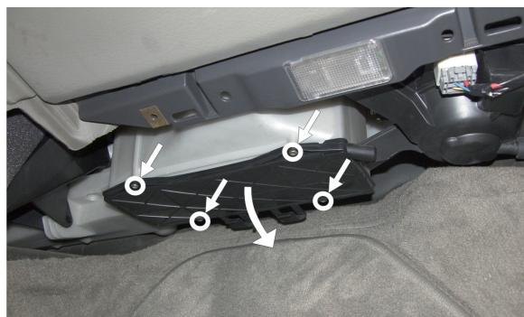
(EN) Loosen the screws that hold the cover itself. Remove the housing
