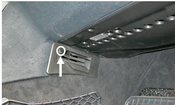
**EN** The filter is located under the glove compartment. Loosen the screw of the air outlet
