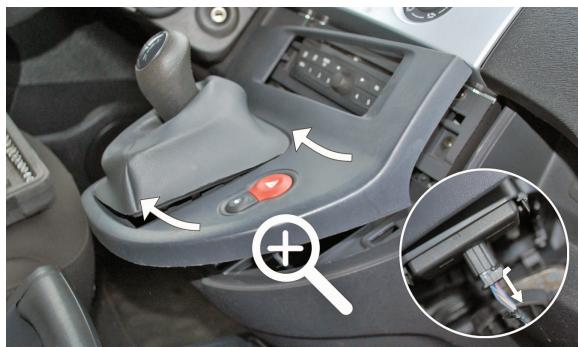
(EN) Remove the element shown in the picture. Disconnect the electric circuit
