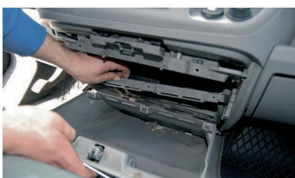
(EN) Filter is located behind the glove compartment
