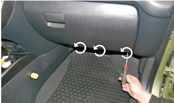
**EN** Filter is located behind the glove compartment. Loosen the screws and remove the glove compartment
