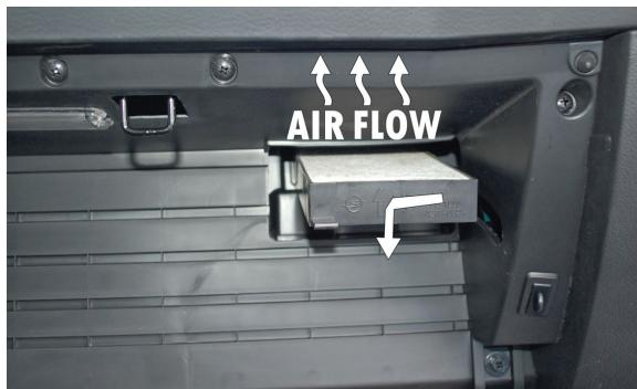
**EN** Carefully remove the second filter, install the new one and perform the previous actions in the opposite order
