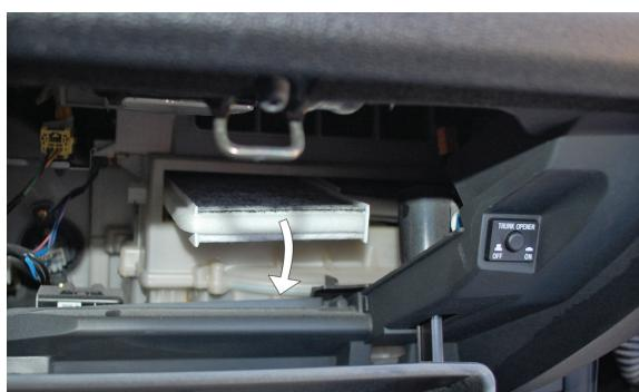
**(EN)** Carefully remove the filter from its socket
