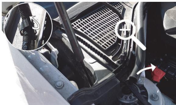
**EN** Remove the rubber seal. Remove the protecting device
