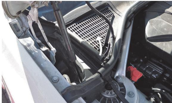
**EN** Remove the rubber seal
