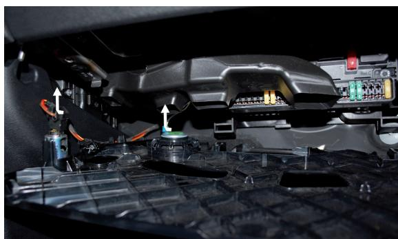
**EN** Disconnect the electric circuit
