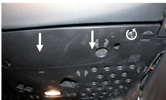
**(EN)** Remove the screw that secures the lower cover of compartment and remove the cover
