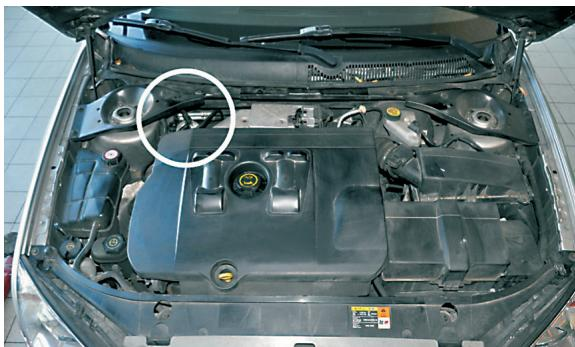
(EN) Clean the area around fuel filter and fuel pipes
