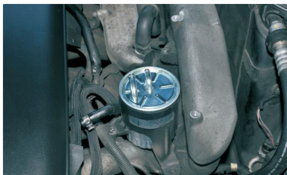
**(EN)** Install new filter, remove safety plug from filter
