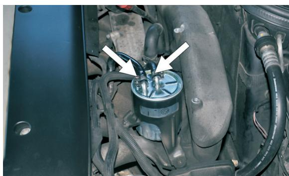
**(EN)** Fasten filter clamping ring, install fuel pipes, start the engine, check system for leakage
