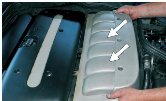
**(EN)** Fix engine casing
