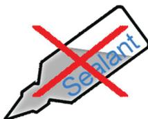
At O-rings, no additional sealant may be used! As an assembly aid an acid-free lubricants like Vaseline should be used. An alternative possibility is to moisten the seal with coolant
