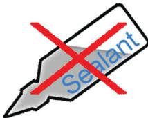
Since the sealing lip in the form ring is sealing, no additional sealant may be used! In order to hold the sealing ring in position, a suitable acid-free lubricant may be used.
