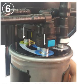
Take the already assembled tubes with the bracket from picture 4 and place them on the filter as shown in picture 6. Make sure the colors of the tubes match the color codes of the filter.
