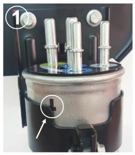
While placing the filter on the bracket, make sure the marker on the filter is placed like it's shown on picture 1.
