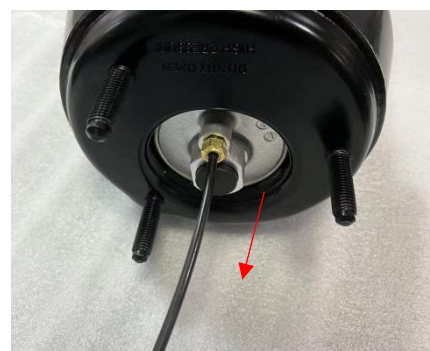
After entering the air line, pull the air line outward to lock and ensure a secure connection
