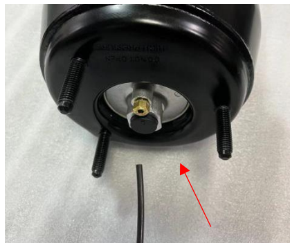
Insert the air line into the connector and press until it is felt to engage
