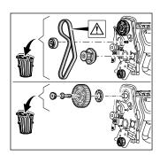
The timing belt must be removed in order to replace the faulty camshaft phasing unit. As the timing belt must be replaced at defined intervals, for economic purposes it usually makes sense to also replace the complete timing belt drive together with the tensioner pulley, the deflection pulley and the water pump. In the event of oil leakage, the timing belt drive must be replaced!
